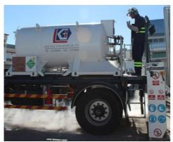
Liquid Oxygen (LOX), is a pale blue, odourless and non-toxic liquid which rapidly evaporates to a colourless, odourless and tasteless gas It is used for big consumption and supply by our cryogenic tank trailer thus reducing cylinder handling
